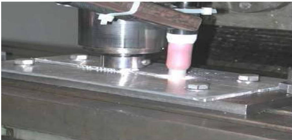
Figure 3-1: HFSW equipment with participation of a GTAW heat source
