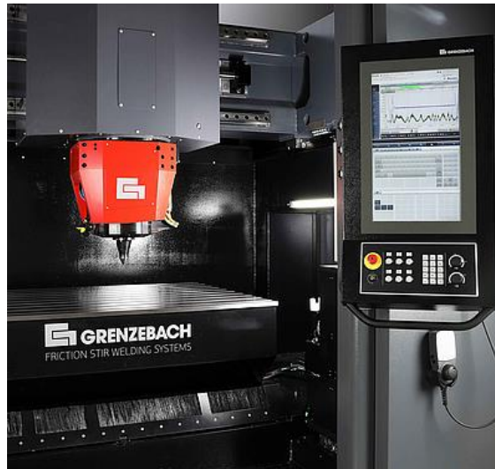
Figure 2-11 Example of machine and control panel (source: Grenzbach)
