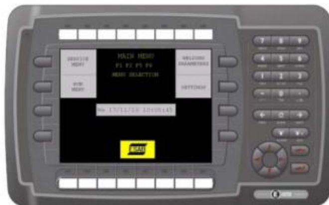
Figure 2-12 Control system developed for FSW (source: ESAB)
